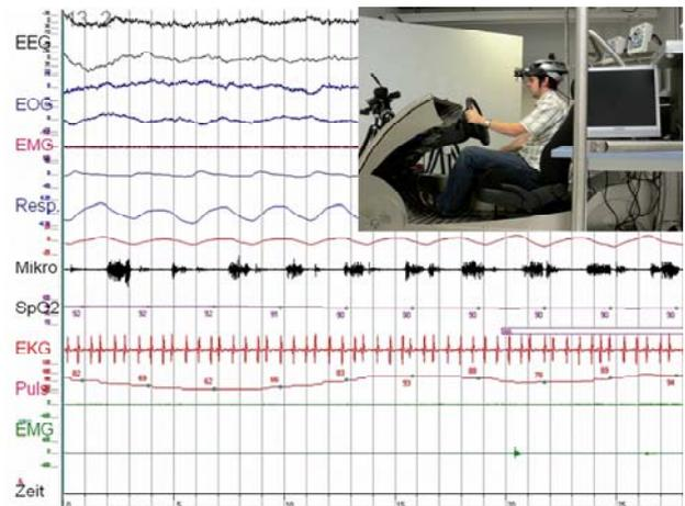
**Figure 4. Simultaneous polygraphic recording of vital parameters.**
