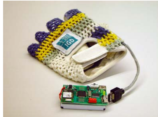
Figure 3. The ERECblue system used.
