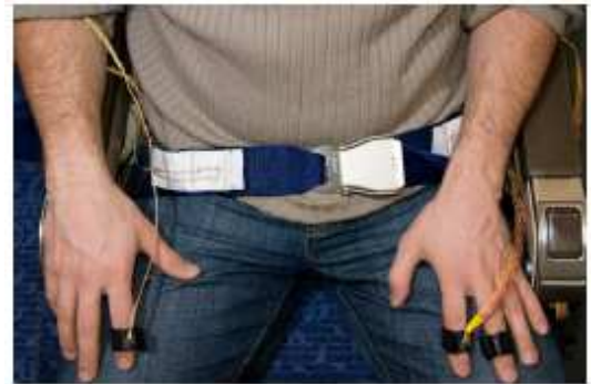
Figure 5. EDA measurement at the left hand, respiration sensor in the seat belt. The additional electrode at the right hand can be applied to measure ECG. It was not used due to technical problems encountered shortly before experiment begin.
